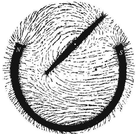
Figure 1.2 Magnetic field lines. The horseshoe magnet SN rotates the compass needle in a counter-clockwise direction.
