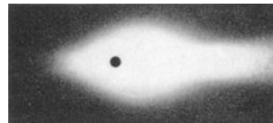
Figure 26.10 The lack of symmetry of the scattered radiation from large sulfur particles: “forward scattering”, along the direction of the primary light beam, predominates (the setup is shown in Fig. 26.9, top; the light used is unpolarized, from an incandescent lamp. This image is about 1/10 actual size).
