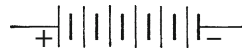
Figure 1.25 A series circuit of 6 batteries. (The positive electrode is always denoted by a longer bar symbol)
