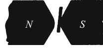
Figure 8.7 Eddy currents brake the fall of a silver coin in an inhomogeneous magnetic field (Video 8.2)
