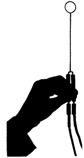
Figure 5.9 Probe coil for measuring the magnetic flux density of an electromagnet (one turn with an area of 3 \text{ cm}^2 ; this corresponds to N_J A = 3 \cdot 10^{-4} \text{ m}^2 ‘area turns’)
