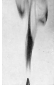
Figure 28.1 A brightly glowing, strongly turbulent flame from natural gas containing benzene vapor casts a deep dark shadow when placed in front of the condenser of a projector
